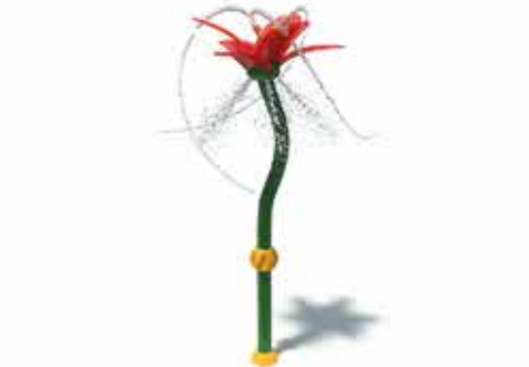
FLORET S-07.18 Dimension (inch/cm) h 118.9-302 w 40-112 Flow Rate 25-35gpm 94-132lpm Pressure 5-10(psi) 0.5-0.7(bar) Spray Zone (inch/cm) 98.4-250
